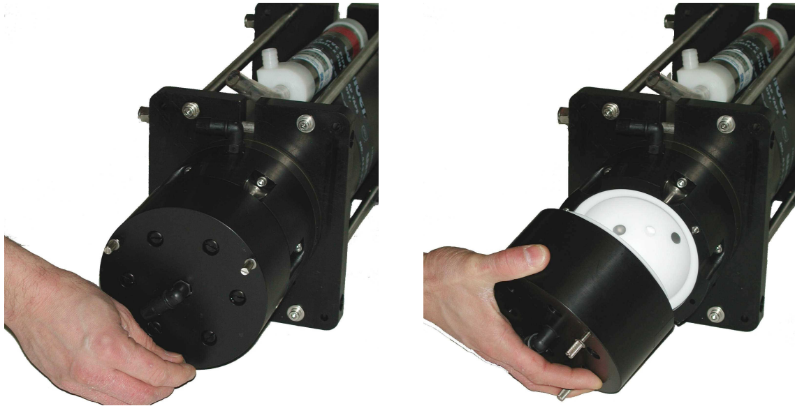
Figure 5. Sphere removal. To open the sphere, loosen the three thumb nuts and gently pull the halves apart. When replacing the removable hemisphere, tighten the screws only by hand.
