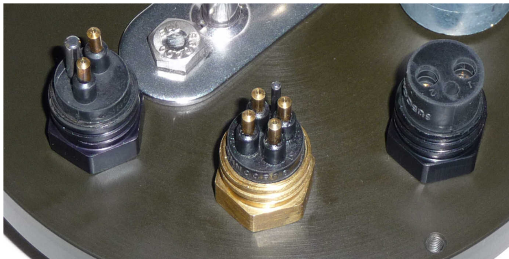
Figure 1. Standard connectors for Series-200 a-Spheres: 2-pin male for power input, 4-pin male for power and data, and 2-pin female for driving a pump.
